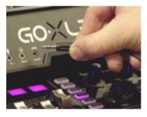
7. If you will be gaming on a Playstation<sup>+</sup> or Xbox<sup>+</sup>, plug these gaming consoles into the OPTICAL output on the rear panel.
